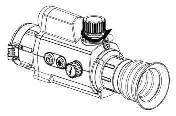
Figure 2-1 Open the Battery Cover
