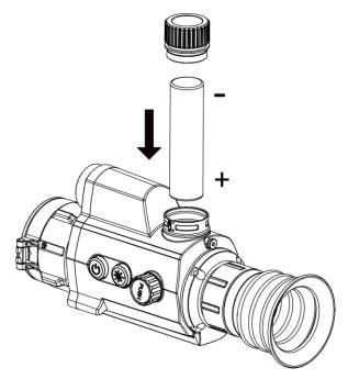
Figure 2-2 Install the Battery
