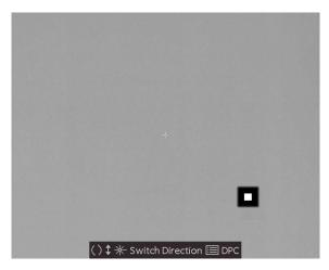
Figure 3-2 Correct Defective Pixel
