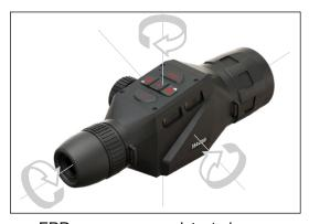
When the compass needs to be calibrated, the word "CAL" appears instead of the Compass Scale. To calibrate rotate the device on three axis rotation, as pictured on the left.
